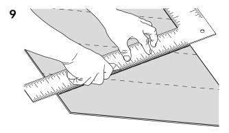
Install the last two 'A' and 'B' planks by cutting the angled end straight to the correct length to go against the wall, taking care to leave the 5mm expansion gap.
