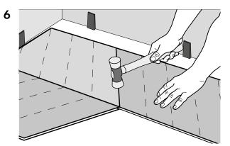
Continue the row by locking another 'A' and 'B' plank into the first 'A' and 'B' plank. Align the tongue of the short side of the next 'A' plank over the groove of the first 'A' plank, ensure the planks are perfectly aligned along the long side and tap the drop lock joint into place using a rubber mallet.
