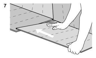
Put the tongue of the next 'B' plank into the groove of the 'A' plank, align the tongue of the short side over the first 'B' plank and tap the drop lock joint into place using a rubber mallet.
