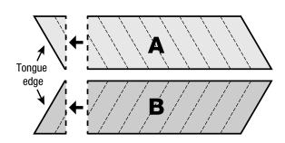
The first 'A' and 'B' planks need the angled end cutting straight as shown to go against the wall. To start the pattern lock the 'B' plank into the 'A' plank along the long edge by putting the tongue into the groove at an angle and dropping flat. Be very careful to align the points of the planks perfectly to ensure the Chevron pattern is correctly aligned.
