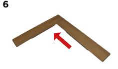
to the perimeter of the installation. direction preferred. Mark a "starting line" on the floor with your pencil. Ensure that you include the 5mm expansion gap when measuring.
