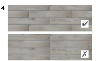
When planning where to start from, ensure that you stagger the joints on each row. There should be at least a 1/3rd of a plank or tile length between each end joint. Do not have all the joints running in a line.
