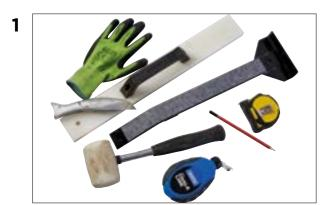
As a minimum, to install Luvanto Endure Pro flooring you will require a utility knife, tape measure, rubber mallet and a pencil. If you use a professional flooring installer, he will have all the right tools for the job.
