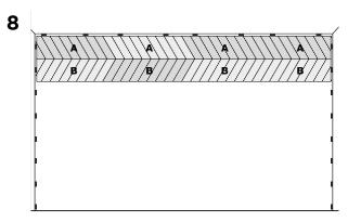
Repeat this for the full length of the row across the room. Always fit the 'A' plank first then the 'B' plank.
