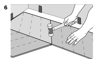
Continue the row by locking another 'A' and 'B' plank into the first 'A' and 'B' plank. Align the tongue of the short side of the next 'A' plank over the groove of the first 'A' plank, ensure the planks are perfectly aligned along the long side and tap the drop lock joint into place using a rubber mallet.
