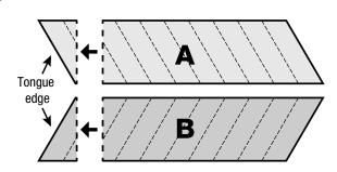
The first 'A' and 'B' planks need the angled end cutting straight as shown to go against the wall. To start the pattern lock the 'B' plank into the 'A' plank along the long edge by putting the tongue into the groove at an angle and dropping flat. Be very careful to align the points of the planks perfectly to ensure the Chevron pattern is correctly aligned.
