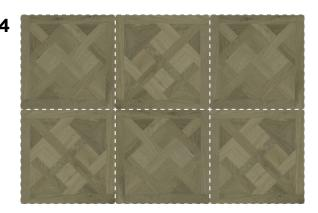
The panels must be laid in straight rows as shown. Do not stagger the joints along each row. All the joints must be perfectly aligned in both directions. We recommend you mix the panels from a few boxes together for best mix of the finished pattern.
