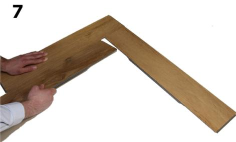
To engage the system correctly click the long sides of the planks together first at an angle then gently slide the planks into position so the short sides are locked into place. You may wish to use a rubber mallet and tapping block to assist with this.
